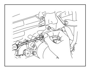
B. With the shaft of the thermostat pressed in, push a pin (diameter 1.0 to 1.8 mm [0.04 to 0.07 in.]) into the hole on the side of the thermostat's cap. Insert the pin until it passes through the hole on the other side of the thermostat's cap to hold the shaft in place.
