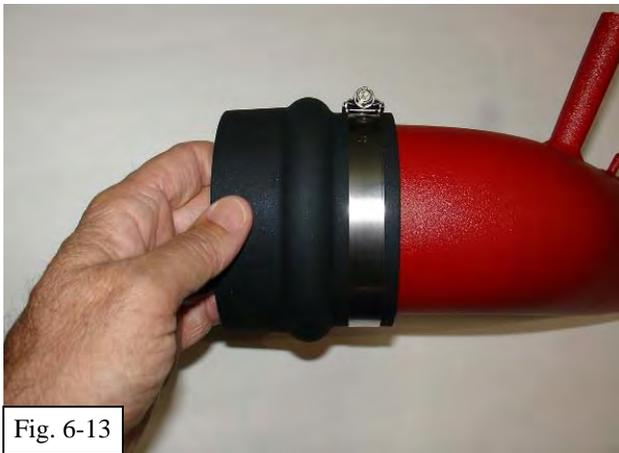
(n) Install supplied 4.0" / 3.5" hump hose on inlet pipe (Fig. 6-13).
