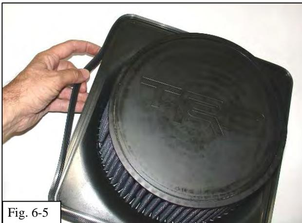
(e) Install OE rubber gasket onto TRD conical air filter base (Fig. 6-5).
