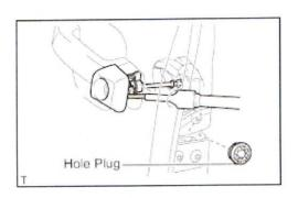
(a) Using a T30 "TORX" socket, install the cover (with the door key cylinder) with the screw.
