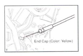
(a) Install the front door lock remote control cable.
