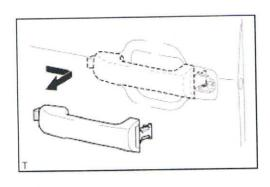
(a) Remove the handle by sliding and pulling it in the direction indicated by the arrow in the illustration.
