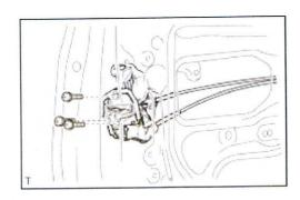
(a) Using a T30 "TORX" wrench, install the door lock with the 3 screws.
