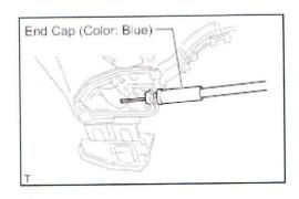
(a) Install the front door inside locking cable.
