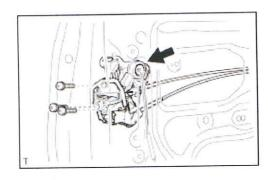
(c) Using a T30 "TORX" wrench, install the door lock with the 3 screws.
