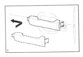
(a) Install the handle by pushing it in the direction of the arrow in the illustration.
