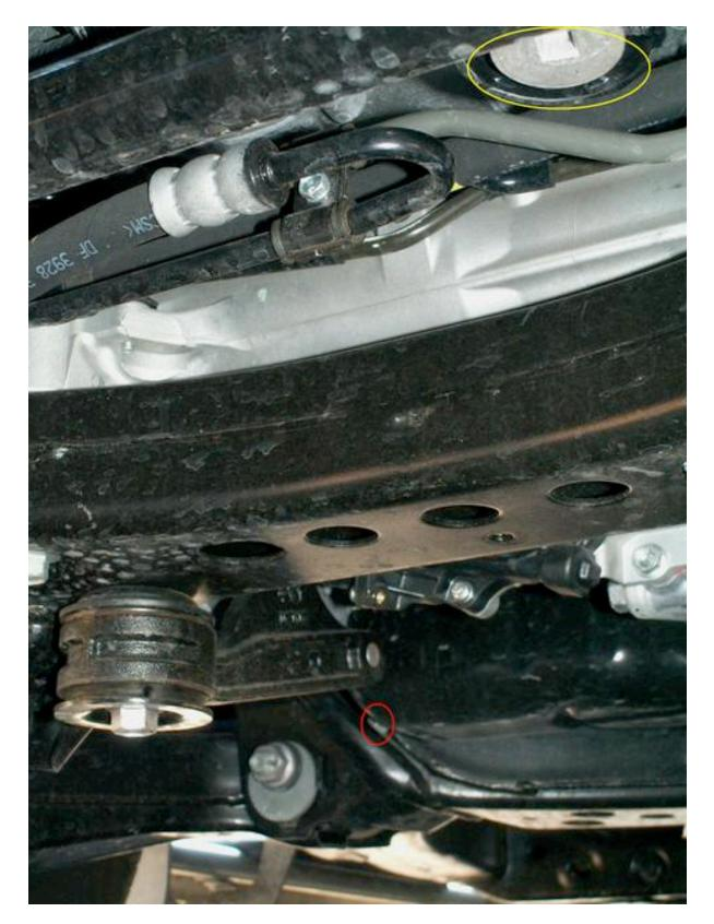
Once you remove the skid, you'll need to identify where the oil filter (in yellow) and bulk oil drain bolt (in red) are located. I've indicated them as pictured above.
