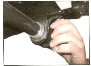
6. Using a 22mm socket, loosen and remove bolts that attach the strut to the lower control arm. Sometimes a pry bar or a slight tap with a hammer is needed to remove bolt- Caution: Try very hard not to damage threads, because this bolt will be re-used. (This view is from the back side of control arm on drivers side of vehicle)
