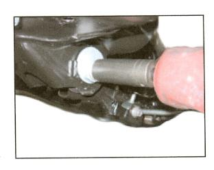
8. Using 14mm wrench, loosen top strut nuts. While holding strut with one hand, remove the 3 upper strut nuts and remove strut from vehicle. Be careful not to tear CV axle boot on 4X4 models when removing strut.
