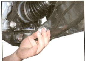
7. Loosen lower control arm bushing bolts (eccentric cam bolts) so lower control arm can swing down.
