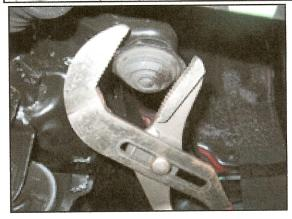
16. Install the two 22mm head lower ball joint bolts starting with the rear bolt first as it is easier to line up with the spindle. Torque to 221 ft-lbf.
