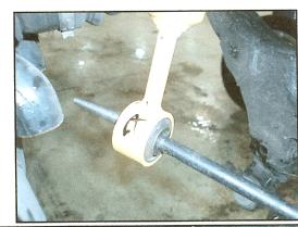
13. Using a jack, raise the lower control arm until the hole on the control arm lines up with the lower strut hole. Install the lower strut mounting bolt and nut and tighten to 144 ft-lbf. A method some use while on a lift
