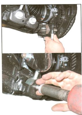
Using a 17mm socket, loosen bolt most forward on the sway bar (has notch in bracket) and remove rear bolt. Remove Sway bar from vehicle.
