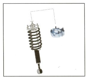
10. Install factory flanged metric nuts and tighten to spacer. Evenly torque each nut (as pictured) in an even sequence to 33 ft-lbf. Sometimes it is hard to hold the strut while tightening the nuts, there is many different ways to combat this- we have found the easiest way to do it is by putting a small pry-bar through the end of the lower strut hole and tighten the nuts.
