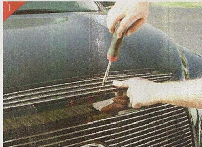
Place the machined grille into opening and center attach using the supplied 10-32 x 5/8" Stainless Steel bolts as shown without over tightening.
