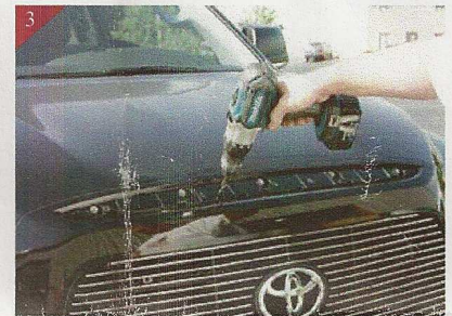
Remove machined grille and drill the just marked hole locations. Drill using a 3/16" drill bit as a pilot hole then move to a 3/8" drill bit and drill again as shown. Repeat process for remaining attachment holes.
