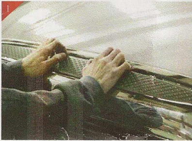
Remove the plastic rock guard from top of stock shell. Do so by unclipping at one end and working to the other.
