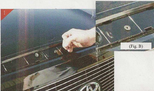
Place the supplied rubber well nuts in just drilled locations as shown. Push in place so that the top portion seats against hood as shown (Fig B).
